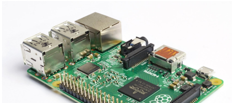
Raspberry Pi 2 ARM Cortex A7 @ 900 MHz Main memory 1 GB (shared with GPU)
