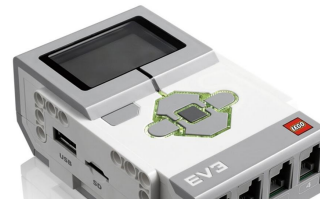
Lego EV3 TI Sitara AM1808 (ARM926EJ-S core) @300 MHz Main Memory 64 MB RAM 16 MB Flash
